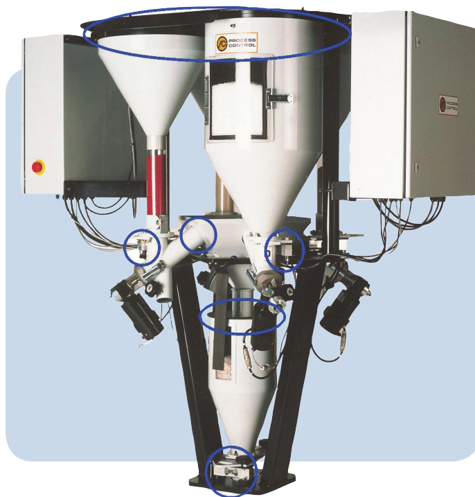
Fig. 2—An X-Series continuous blender, showing inspection points (circled) for potential weighing system interference.
