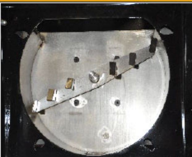
No Dead Space Mixing Chamber With Welded Single Piece Scroll
