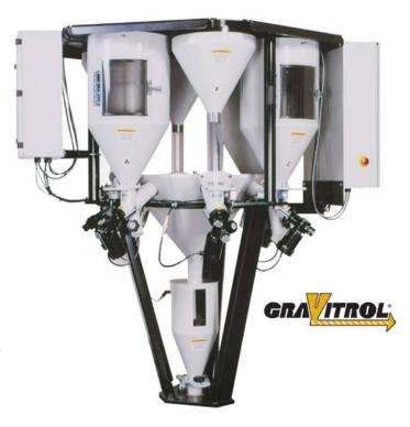
With the new on-line blending capability, in addition to gravimetric control of both the puller and extruder, the materials feed and total line yield were now fully automated and accurate to within +/- 0.5% by weight. This resulted in faster line start-up, reduced overall scrap and improved product quality. Gunther and Jon were successful in adding a significant level of automation and process improvement to the line, with a minimal capital expenditure and utilization of surplus equipment.
