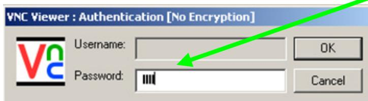
Click OK to log on to the blender touchscreen. You now have full control of the machine just as if you were standing in front of it. The mouse cursor looks like a small black dot. To exit the viewer click on the X in the top corner. Note that this will not shutdown the blender.
