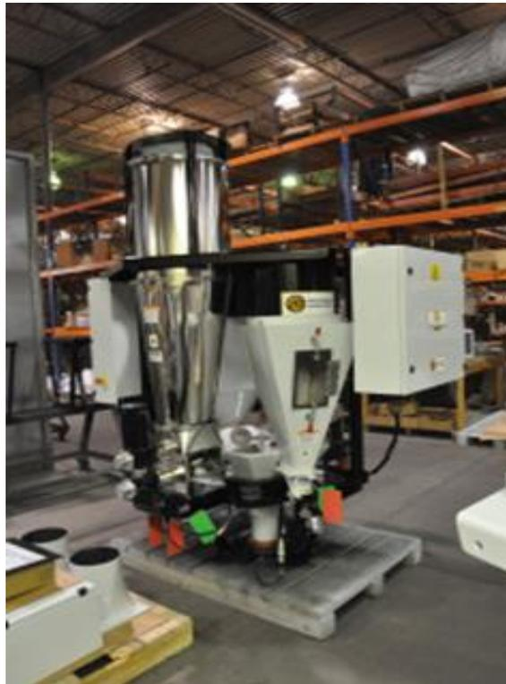
Shown in picture above, a configuration with an extended hopper. [Follow the link](#)
